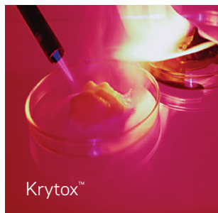
Hydrocarbon-based lubricants burn; Krytox™ does not.
